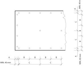
Required distances as a function of the most frequently used board thicknesses
